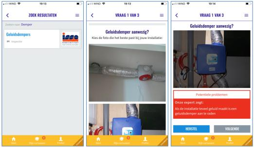
Image 5: Impression of the 'Inspection Interaction'
